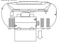
2. Fit two 'C'/'UM2' batteries into the lower battery compartment, observing polarity as shown.
